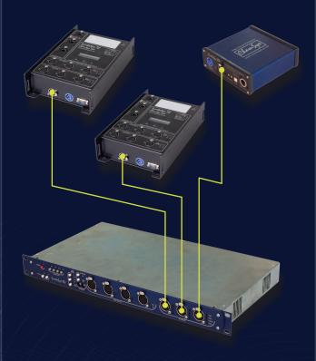
Typical configuration. SnakeSys R4 powering SnakeSys B4 and SnakeSys T2s, remotely configured by MagicQ console via the ChamNet protocol.
